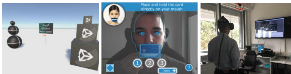
Figure 8. Study setup. (left) VR tutorial level; (center) interpupillary distance measurement (IPD tool); (right) room-scale setup for the study
