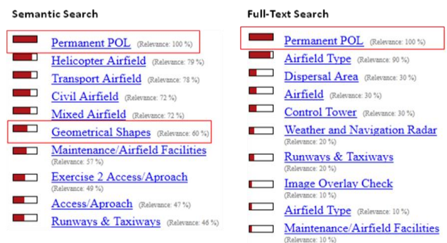
Figure 6. Results of semantic retrieval (left) and full-text search (right). The filled bars on the left indicate the relevance of an entry
