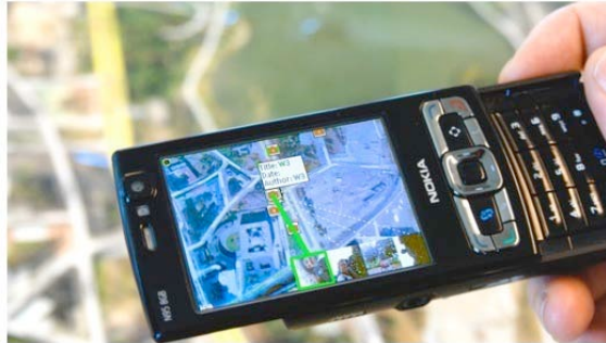
Figure 1: The MapLens application showing a live video of the paper map underneath, augmented with icons and labels registered to map locations.
