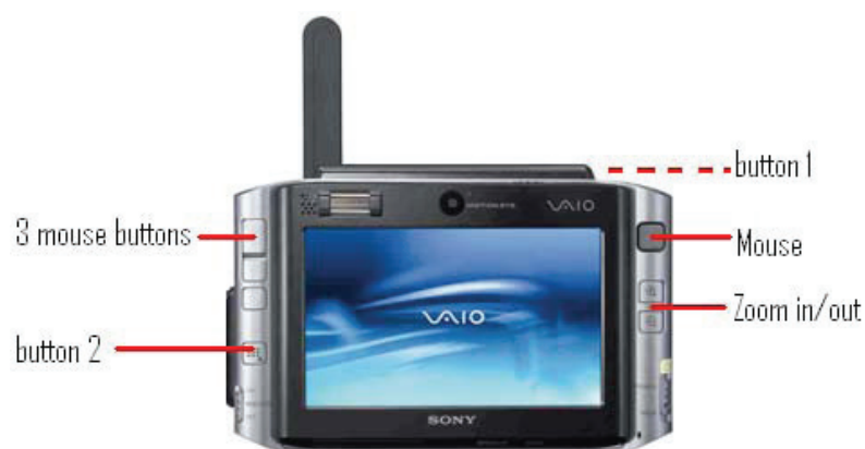
Figure 1 An Ultra mobile PC was used as mobile AR system for the year 3 prototype.
