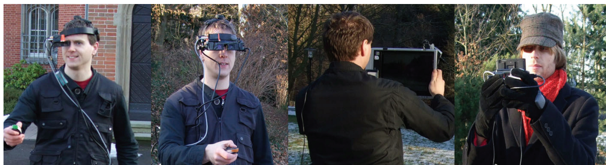
Figure 6 Compared devices: monocular and binocular see-through display (left) and Tablet PC and UMPC (right).
