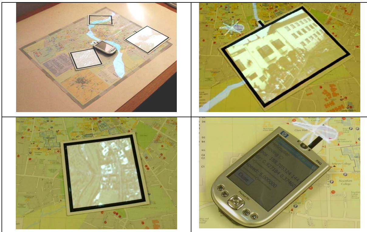
Figure 29 - (Top left) Overview of the augmented map system. The demonstration setup shows the river Cam flooding surrounding areas in the City of Cambridge, UK and related information. An image browser (top right) provides access to geo-referenced pictures, while a satellite view (bottom left) shows a different layer of data. A PDA-based tool (bottom right) displays a remote user interface to communicate with a helicopter.
